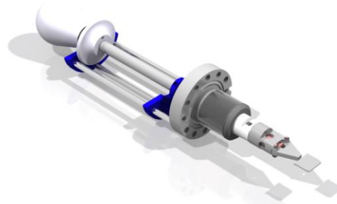
Fig 14 Wide angle wobblestick with a TSWM and a PGWMS(OM) clamping a flag style sample plate
